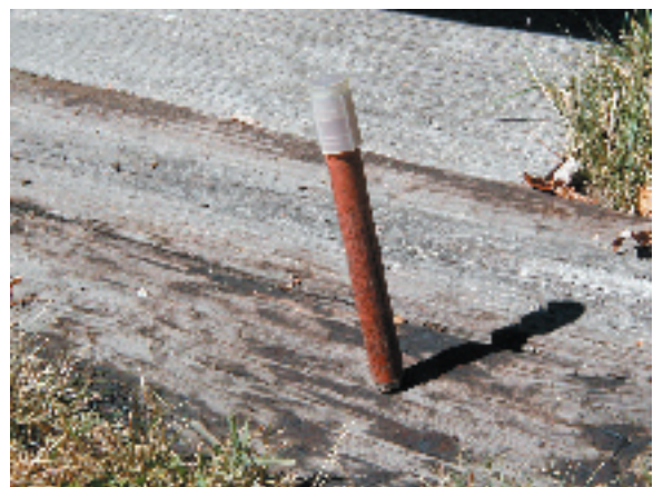
Fusee, or flare--used for warning crews of other trains of various emergencies; in common use by railroad crews (Cap contains igniting device.) Phot by Eugene Smith
