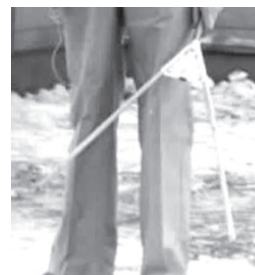
Closeup of train-orders hoop (used before days of electronic train control)
